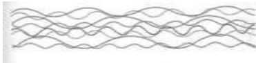
◀ Figure 31.25 Incoherent white light contains waves of many frequencies and wavelengths that are out of phase with one another.
